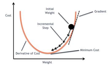
Intuition: Negative gradient is the steepest decreasing direction at that point. So if the step size is small and the function is convex, the algorithm will reach the minimizer.
